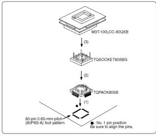
Figure 3 Connecting procedure
